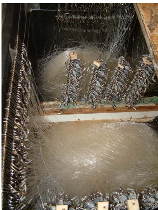
Figure 7 Hooks, snoods and swivels, stowed in a large bin, ready for deployment
