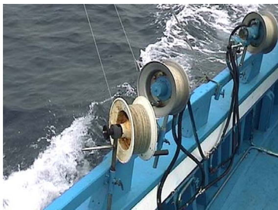
Figure 11 Example of a hand-operated reel (lower centre) alongside hydraulic-powered reels
