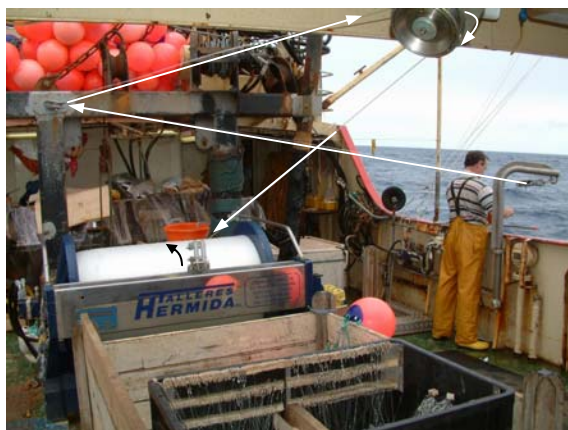
Figure 9 Hauling the longline, showing the path of the nylon monofilament
